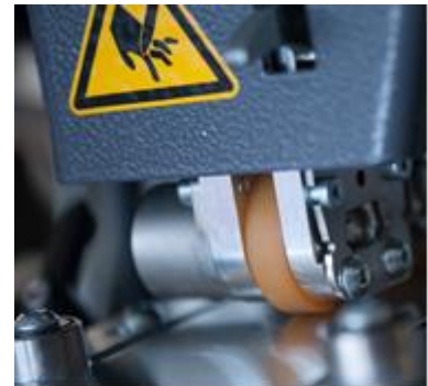
To provide feedback regarding the actual position, tecodrive uses two high-precision and very light measuring wheels, which can also detect any potential slippage.
