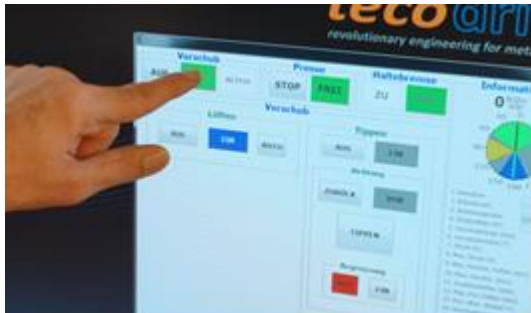
The flexcontrol operator interface for the feed unit. Punching is made easier by inching the strip forwards and backwards within a restricted section of feed length
